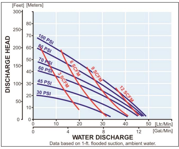
To calculate performance for Santoprene® and Hytrel®-fitted pumps, use Rubber Diaphragm Curve.
